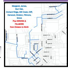
The Public works Department will be cleaning sewer lines during the month of April. A cleaning nozzle is propelled from one manhole to the next using water under high pressure. The nozzle is then pulled back to the starting manhole. As the nozzle is pulled back, water scours the inside of the sanitary sewer pipe. Any debris in the pipe is pulled back with the water. If roots are found, they are cut with a root cutter. This process is repeated on every sewer line cleaned.
